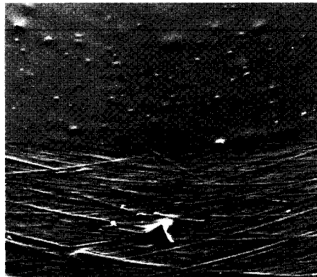
Fig. 23. CANNULA, arterial at tip, polyvinyl chloride: smooth-rough junction; polishing process has removed perpendicular ridges but leaves numerous smooth-edged blebs (100X)
