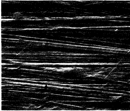
Fig. 15. MICROEMBOLI FILTER, housing, polypropylene: uniform surface; many large ridges perpendicular to blood flow; occasional small, smooth-edged pits; occasional small scratches crossing ridges (1000X)
