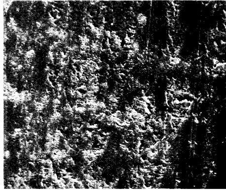
Fig. 1. CANNULA, venous, polyvinyl chloride: uniform surface; gentle indentations and low ridges; generally smooth (500X)
