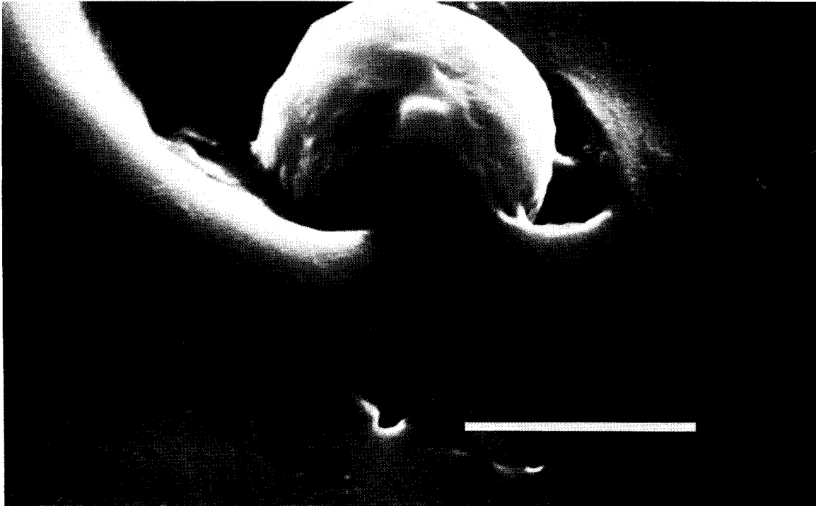
FIGURE 11. Clinically used silicone rubber tubing. Same sample as Figures 9 and 10 but at a higher magnification. Note partially eroded particle within a crater that measures approximately 12.5\ \mu\text{m} in diameter. Bar = 10\ \mu\text{m} .
