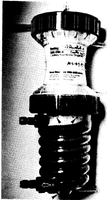
FIGURE 7 - Heparin surface coated hollow fiber membrane oxygenator rinsed after 24 hours cardiopulmonary bypass without systemic heparinization. Note clean oxygenating section (no dark occluded hollow fibers) and clots in heat exchanger section of the device.
