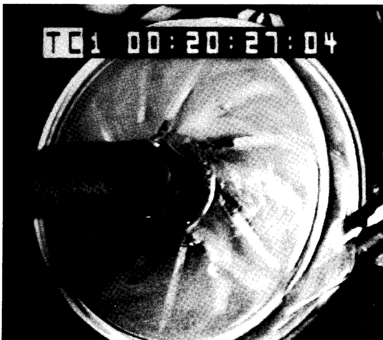
Figure 2 127 seconds after the first evidence of thrombus formation, massive cotton-like thrombi prevent any further forward flow in the Sarns Delphin. A string of thrombus may be seen extending back from the pump for several inches.
