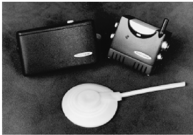
Figure 3: Wearable components: external battery, biotelemetry monitor, and external energy and information transfer coil.
