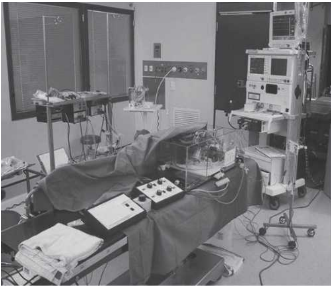
Figure 2. Simulator on operating table connected to CPB machine in the background.
