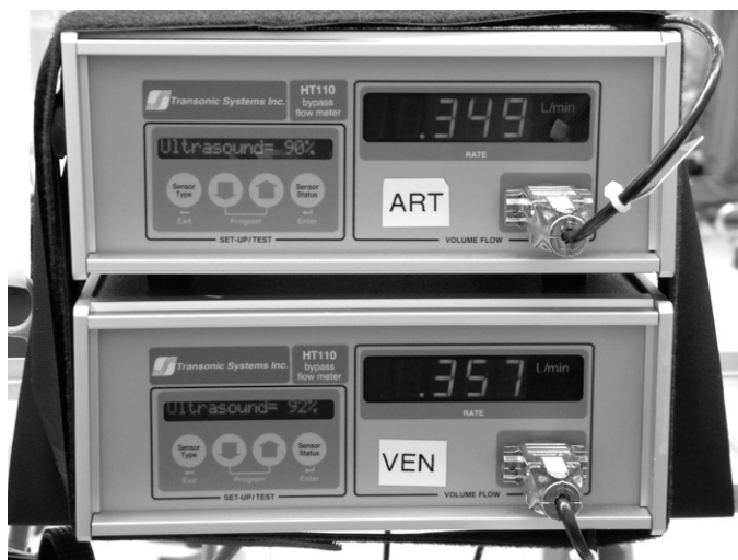
Figure 2. Arterial (top) and venous (bottom) H7XL ultrasound transit time flow probe transducers (Transonic Systems, Inc., Ithaca, NY). “Ultrasound %” displayed shows the amount of ultrasound signal being transmitted based on the manufactured specifications. Small changes in signal quality can be improved by adding ultrasound gel to enhance the transmission of the sound wave. A greater than 10% loss in transmission quality may require the device to be recalibrated.
