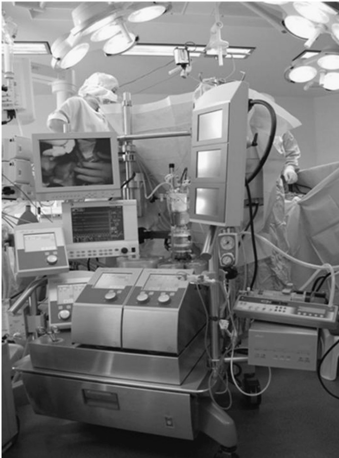
Figure 2. Two-level heart–lung machine: the top of the cardiotomy reservoir is at the level of the patient's right atrium.
