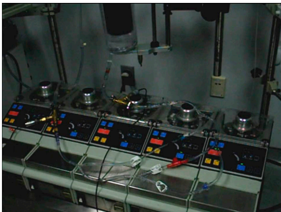
Figure 2. Pressure and flow testing setup.
