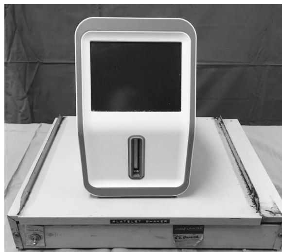
Figure 2. TEG ® 6s on platelet agitator.
