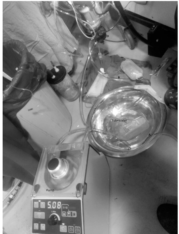
Figure 1. Setup for rewarming without a heater/cooler machine. A: Temperature probe in water, B: Outlet pipe of heat exchanger, C: Inlet pipe of heat exchanger, D: Heat exchanger.
