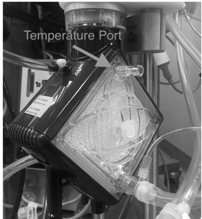
Figure 3. Temperature port of the rotaflow oxygenator.
